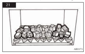
6.18 Place six small coals along the rear of the flame baffle, resting against the rear ledge, see diagram 22.
